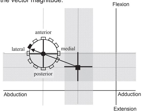
**Figure 1:** Scheme for electrode selection and stimulus intensity. The cross with the square represents the mean and standard deviation of normal sagittal and coronal hip angles at an instant in the gait cycle. The cross with the circle represents the patient undergoing training. For clarity a reduced number of electrodes are shown.
